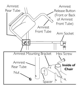
**FIGURE 5.1** Using or Replacing Flip-Back Armrest (Lightweight Wheelchairs Only)
